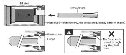
② Make sure that the flared ends engaged the flange, and then use a hammer to strike the tool head and taking out the right cup.
