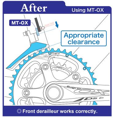
MT-OX allows lower FD mounting to accommodate OX901D compact rings. Proper FD position helps you to get the most performance, comfort and safety.
