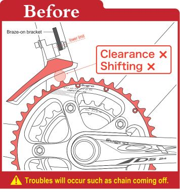
FD cannot be adjusted low enough. If gap between FD and outer ring is too wide, FD won't work correctly. It may cause damage to other parts and even result in serious accidents.
